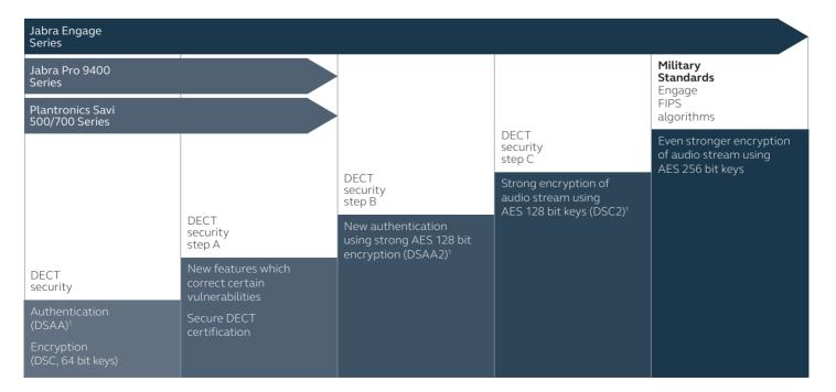
DSAA and DSC are the authentication and encryption algorithms defined in the DECT security standard ETSI EN 300 175-7 applicable for DECT security and DECT security step A. DSAA2 and DSC2 are the equivalent updated security algorithms for the next steps of DECT security, steps B and C.
